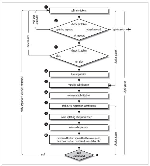
Figure 7-1. Steps in command-line processing
