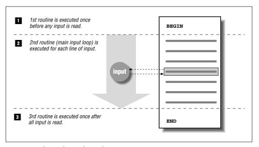
Figure 7-1: Flow and control in awk scripts
